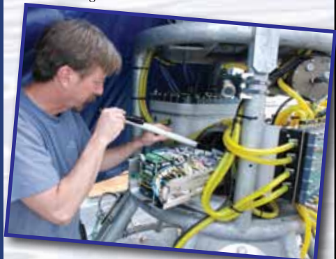
Testing the water leak detector on the Okeanos Explorer 's ROV camera platform. Image credit: NOAA.
