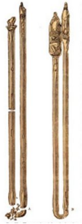
The pressure of the deep left these thermometers broken.
