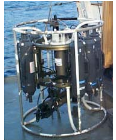
A hydrocast: a CTD with Water Sampling Bottles on a Rosette
