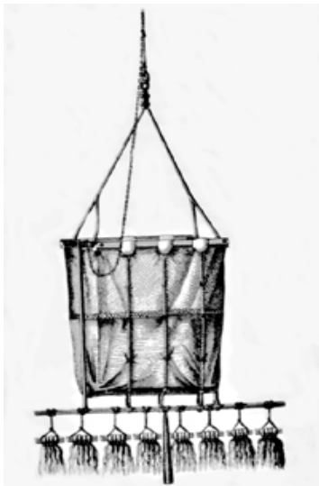
Challenger's Shallow Water Dredge
